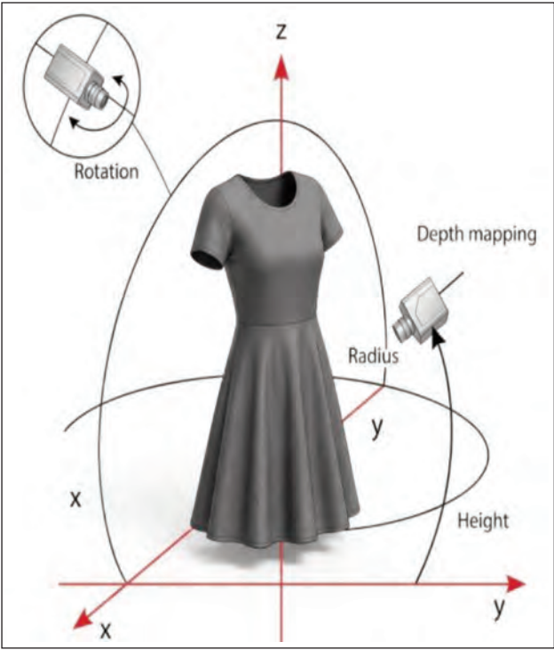
Fig. 2. Fabric depth mapping configuration
