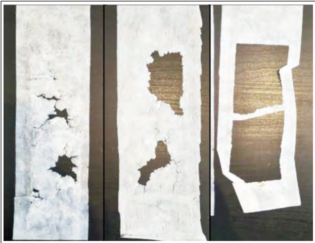
Fig. 4. Post-ageing images of non-woven fabric samples N1-5-4 (200 hours), N1-5-5 (300 hours), and N1-5-1 (500 hours)
